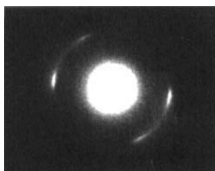
FIGURE 2 Electron-diffraction pattern from a ten-layer FTE1 film in the Sm-L/Sm-C phase at 70.3°C.
